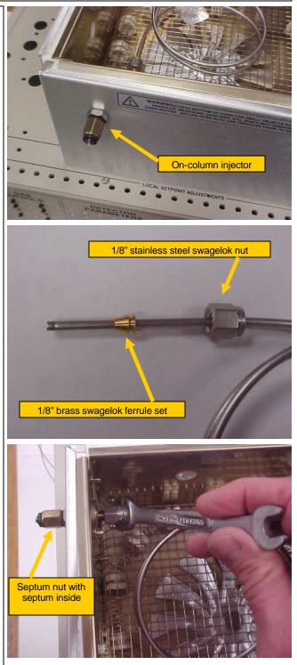
Bend the column gently so it lines up with the detector bulkhead fitting. Attach a stainless swagelok nut and brass ferrule set to the end of the column. It's a
