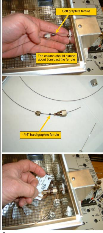
To install a narrow-bore capillary column in the on-column injection port, connect the narrow-bore to a 5 meter length of .53mm MXT pre-column. The precolumn is de-activated MXT tubing but there is no phase coated on the inside of the tubing like a normal column, so analytes are not retained.
