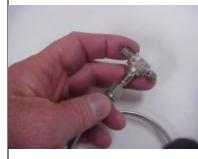
good idea to first tighten the nut and ferrule into a standard swagelok fitting so the ferrule is positioned at a
