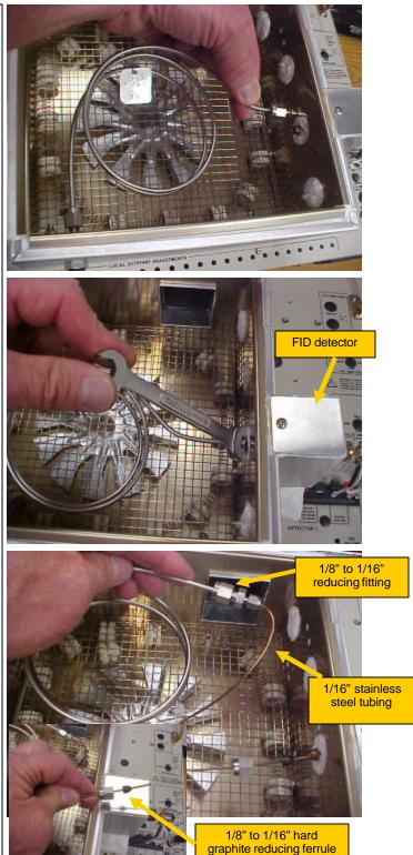
To install a .53mm capillary column in the on-column injector you will need two 1/8" swagelok nuts, two 1/8" to .8mm soft graphite reducing ferrules, the SRI wide bore column adapter, a triangle file to cut the column and a 7/32" wrench.
