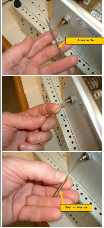
Pull the adapter back into the on-column injector.
