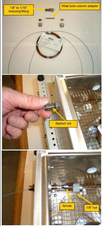
Use a sharp triangle file to cut a few centimeters from the end of the MXT column. It is a good idea to ALWAYS trim the end of the column anytime you run it through a graphite ferrule as the sharp edge of the column can shave graphite off into the bore of the column where it can cause the peaks to tail. Support the column with your fingertips and drag the file firmly across the tubing in one swift motion.
