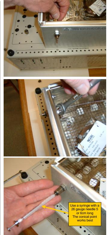
Connect the other end of the column to the detector. The simplest way is to use a 1/8" swagelok nut and a second 1/8" to .8mm soft graphite reducing ferrule. The detector shown in the photo is the FID detector. The end of the column should be positioned about 3cm past the ferrule or about halfway from the inlet fitting to the tip of the FID jet.
